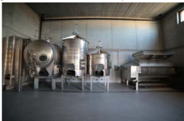
Fig.: 2. Equipment of a modern minimalist in wine making - press & mash tanks
